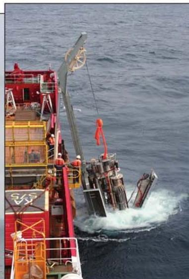
*Deployment of the Prod seabed drilling unit at the Luva location in the Norwegian Sea.*
